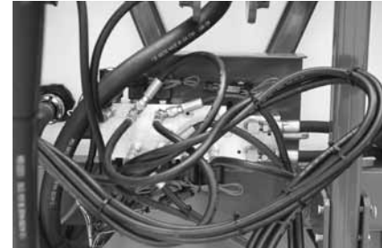
Directional Stack Hydraulic Controller closed center hydraulic system set up, rear view
